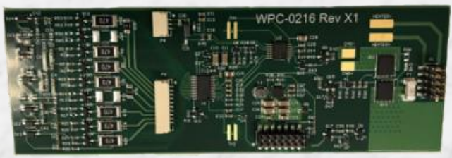
Core pack heating in less than 20 minutes to +5°C from -20°C
